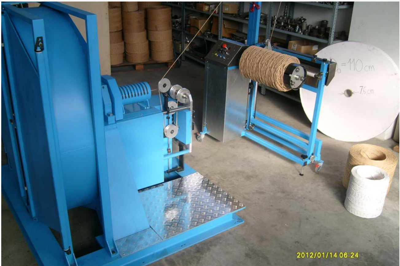
Photos of M09 system: (on the left the Twister Unit, to the right the Winder Unit)
